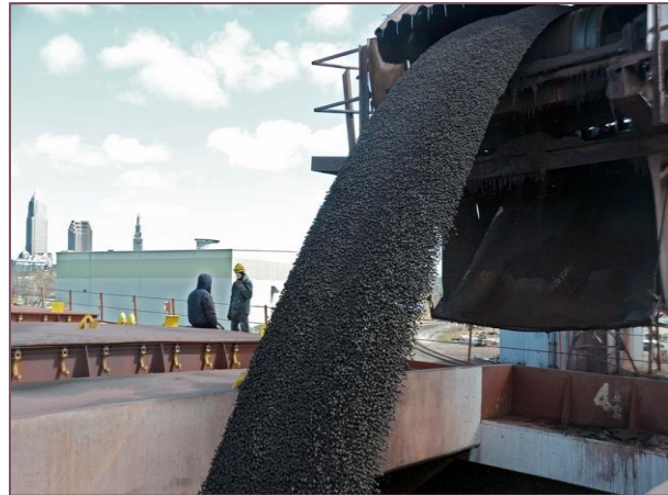
Discharge from conveyor to shuttle
