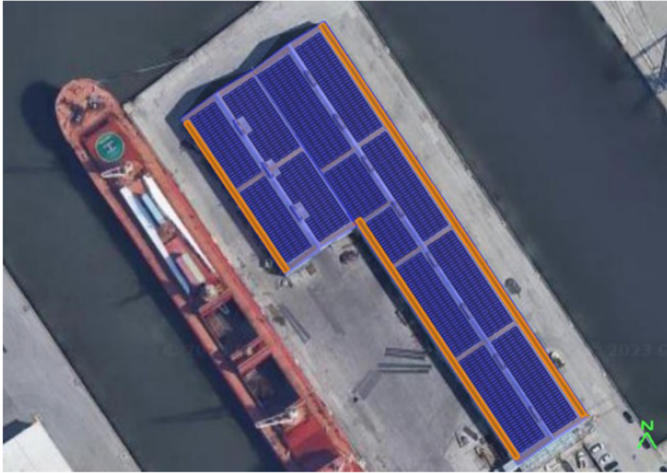
Figure 9-11. Rooftop Solar Helioscope Solar Model-Warehouse 26
