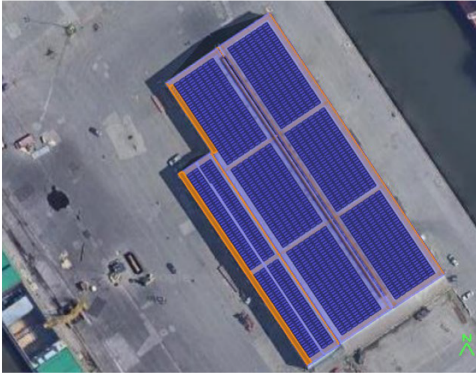
Figure 9-8. Rooftop Solar Helioscope Solar Model-Warehouse 24
