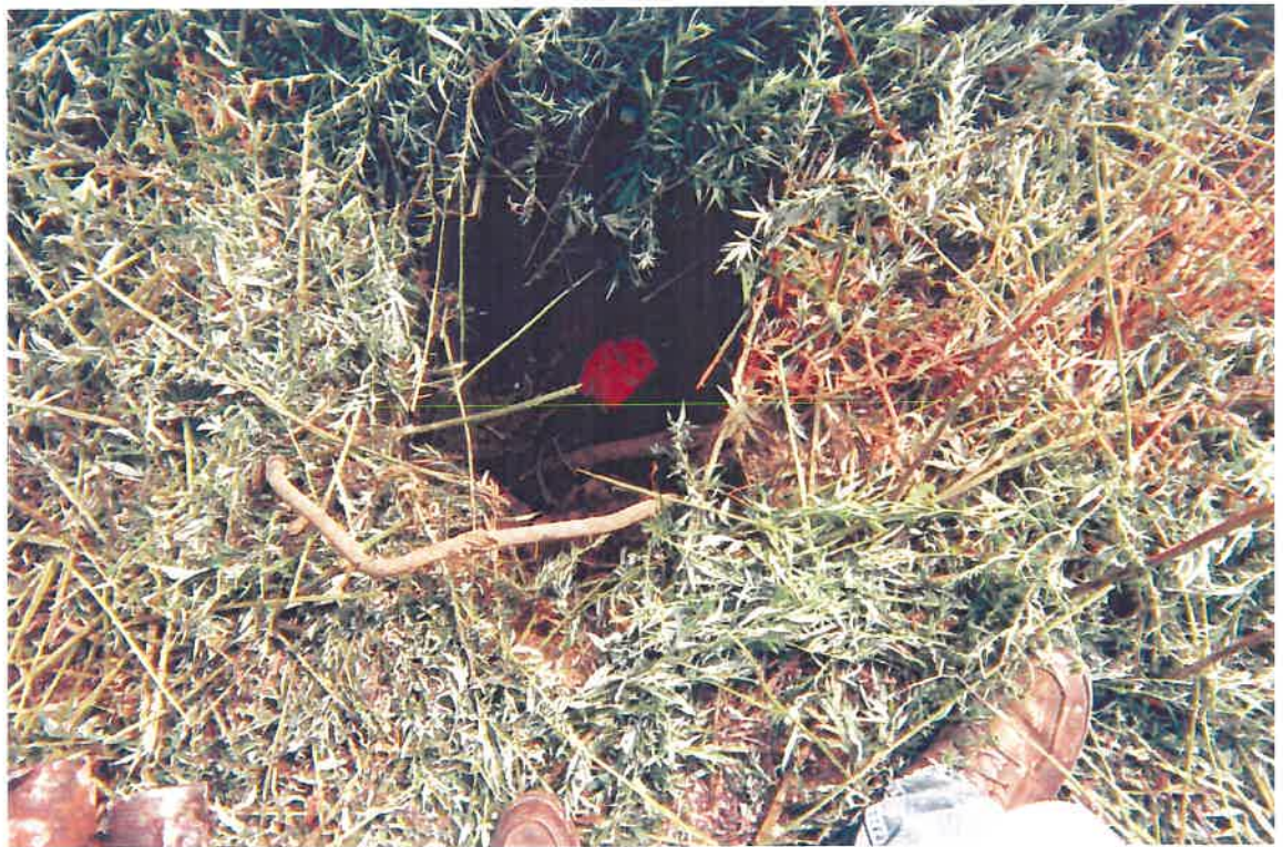
Photo 4: View of boring WC-1 at completion of drilling. Note the steel pipes, large rock and other miscellaneous debris in upper portion of hole.
