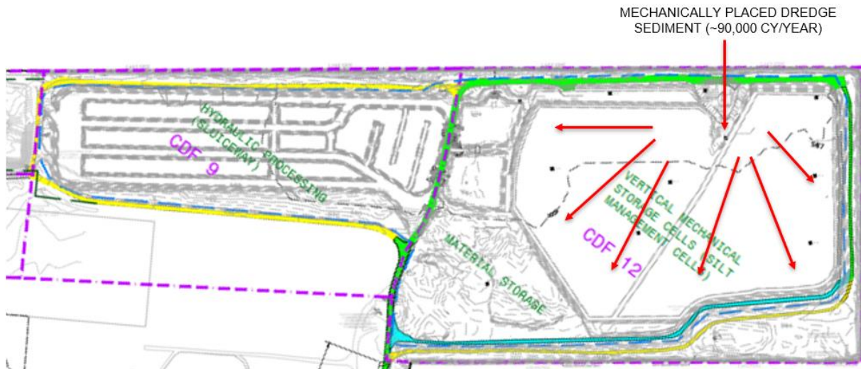
Figure 3. Mechanical delivery of dredge material operating model.
